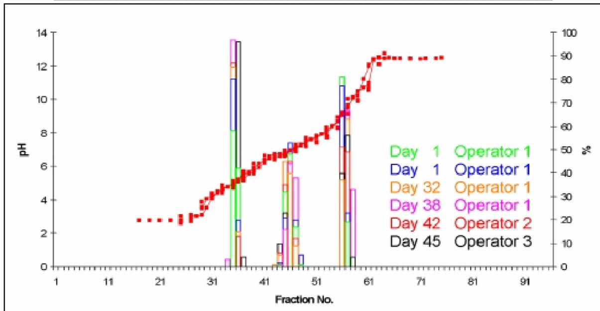
Figure 2: Excellent long-term fractionation-reproducibility of FFE: Superposition of 6 FFE-fractionations of trypsin inhibitor (left peak cluster), carbonic anhydrase B (central peak cluster), and cytochrome C (right peak cluster). pH-gradients: red squares.
